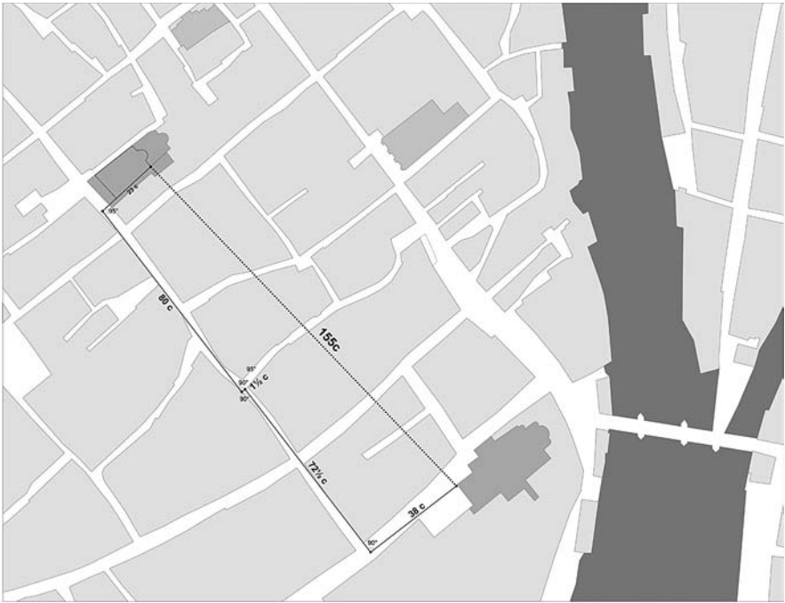
18.1 | Map (scale of 1:1000) showing the measurement in 1327 of the distance between the churches of Santa Maria della Scala (top left) and San Fermo (bottom right) in Verona. The dotted line indicates the distance “per aerem” between the two churches; one canna ( c on the map) is 1.9465 meters. Drawing by Emanuele Lugli and Fernando Lugli.
